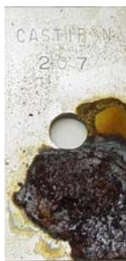
Corrosion attack on cast iron
